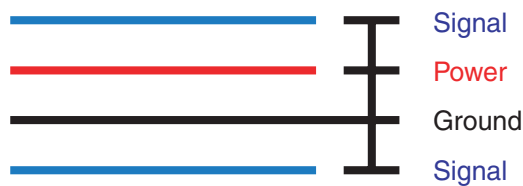
Figure 5-4: Guard ring in a 4-layer PCB
